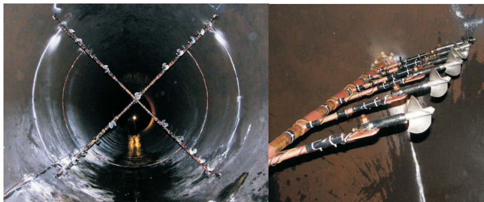
Figure 9: Current-meters and the Gibson method impulse tubes in the penstock of Zur hydropower plant.
