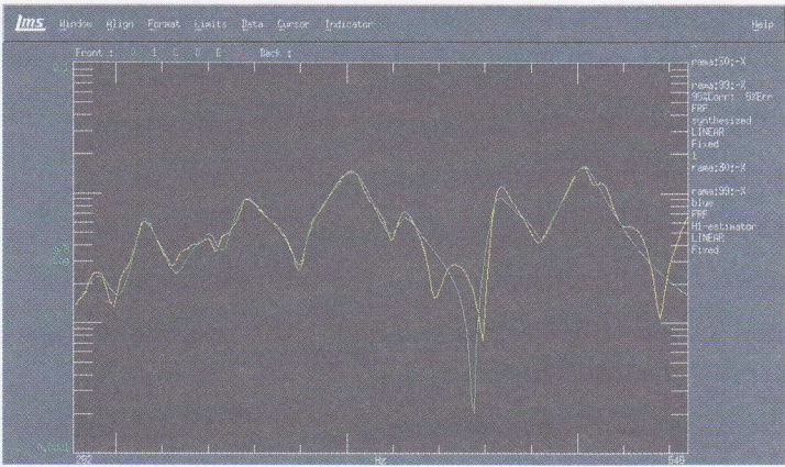
Figure 7. Comparison of measured and determined during analysis distributions of spectral transition functions in the range 282-548 Hz.
