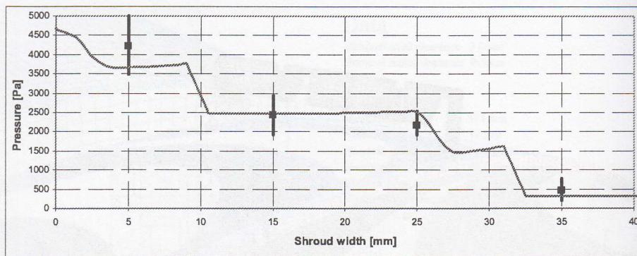
Figure 4. Pressure distribution along the shroud width ( \omega = 566 rad/s), solid line – average pressure calculated by means of MRF method, bars – range of pressure changes according to experimental data.
