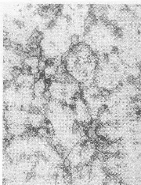
Fig. 3b. The structure of the pad created by means of the EN10-10B electrode – 0.5 mm beneath the cavitated specimen surface. Magnification 280x.
