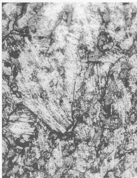
Fig. 1a. The structure of the pad created by means of the IMP 6 electrode – the surface layer of a not cavitated sample. Magnification 280x.
