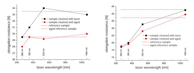
Fig. 2. The dependence of the elongation resistance on irradiation wavelength for the paper samples produced of cotton cellulose and wood –paper mass, with no glue (a) and seized with a resin glue (b) after pulsed laser irradiation at 266, 355, 532, and 1064 nm, and after aging
