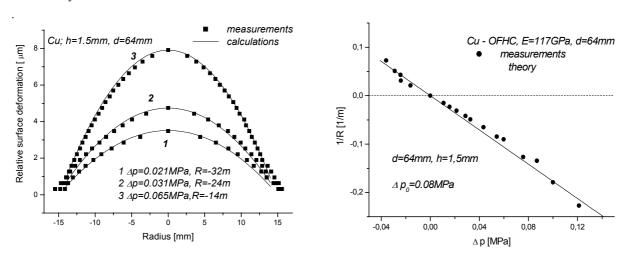
Rys3 2D—contour of the mirror surface resulting from the interferometer measurement (a), the dependence of the curvature radius on the deforming pressure measured in relation to the atmospheric pressure (b)
