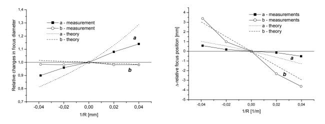
Fig. 4 Focus shift and relative changes in the focus size vs radius of curvature of the variable focal length mirror. The measured values are given in relation to the focused beam waist position and its size for the flat mirror; a – the mirror located at the distance of 0.3m from the laser output window, b - the mirror located at the distance of 0.2m from the focusing lens and 4.2m from the laser output
