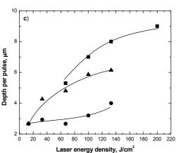
**Fig. 1.** The dependence of the hole depth per pulse in: a)  $Al_2O_3$ ; b) AlN; and c)  $Si_3N_4$  on the laser energy density for different wavelengths.  $\blacksquare$  -  $\lambda$  = 1064 nm,  $\bullet$  - 532 nm, and  $\blacktriangle$  - 355 nm, respectively
