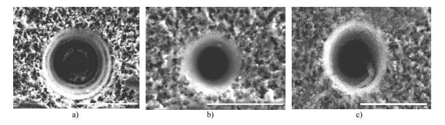
Fig. 3. SEM images of the holes drilled in  $Si_3N_4$  by: a)  $\lambda = 1064$  nm; b) 532 nm; and c) 355 nm laser radiation. The laser energy density is 133 J/cm<sup>2</sup>. The white marks represent 50  $\mu$ m.
