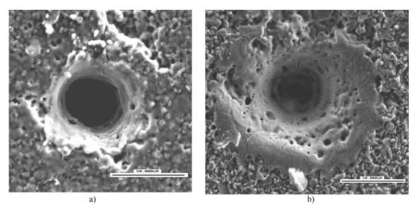
Fig. 2. SEM images of the holes in: a) AlN and b) Al<sub>2</sub>O<sub>3</sub>, drilled by 1064 nm laser radiation. The laser energy density is 133 J/cm<sup>2</sup>.
