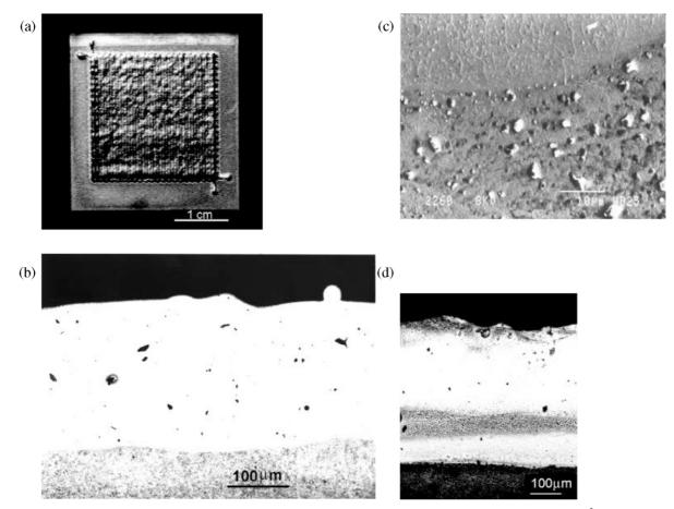
Fig. 2. (a-d) Photographs of the sample structure: a general view of the stellite coating of dimensions  $20 \times 20 \times 0.7$  mm<sup>3</sup> (a); cross-section of a single-layer coating (b); SEM micrograph of the dendritic structure of the stellite (upper zone) and the structure of the substrate; the interface and also white precipitates are clearly observed (c); and a cross-section of a stellite clad, total height of two layers = 0.7 mm, magnification (d).
