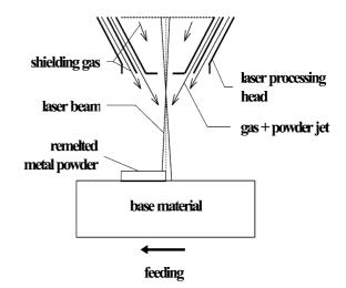
Fig. 1. The axially-symmetric experimental setup applied for the laser cladding of stellite powder.
