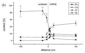
Fig. 3. (a,b) Semi-quantitative EDS data on the dominant chemical components of the bulk stellite-full line, and of its region close to the base material-dashed line (a); dependence of the relative content (%wt.) of constituents Fe, Co, Cr, and Ni on the distance from the substrate-clad interface (b).
