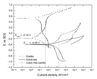
Fig. 6. Dependencies of the electrochemical corrosion potential with respect to the saturated calomel electrode (SCE) on the current density for the substrate (solid line), the laser-clad stellite layer (dots), and for the defect-free reference layer (squares).
