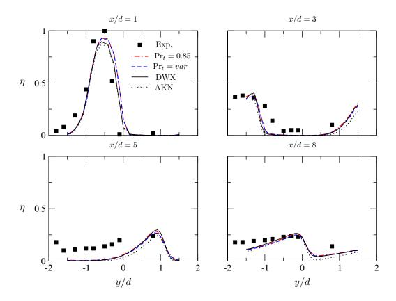
Figure 6. Cooling effectivness for velocity ratio VR = 1.5
