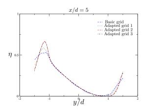
Figure 3. Cooling effectivness  $\eta$  at the cross-section x/d=5 after subsequent grid adaption
