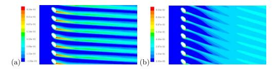
Figure 7. Distribution of cooling effectivness, (a) VR = 0.5 and (b) VR = 1.5
