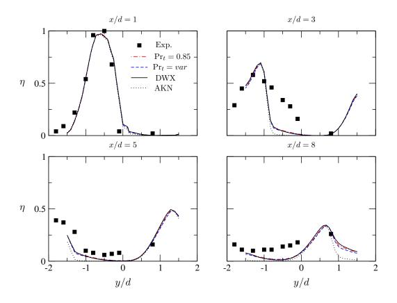
Figure 5. Cooling effectivness for velocity ratio VR = 1.0
