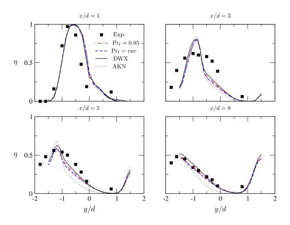
Figure 4. Cooling effectivness for velocity ratio VR = 0.5
