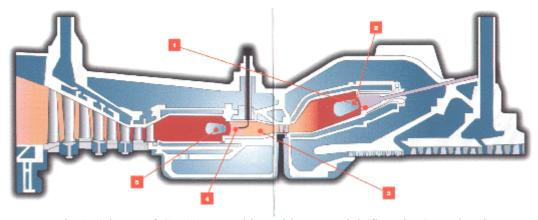
Fig 4. Scheme of GT 26 gas turbine with sequential (flameless) combustion
