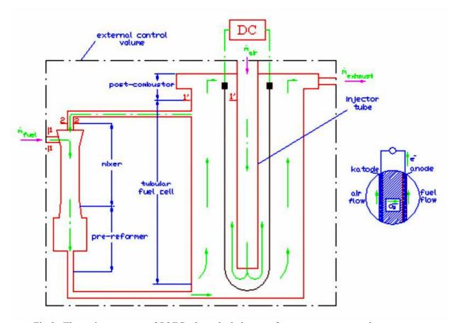
Fig 8. The main apparatus of SOFC where the balances of mass, momentum and energy are executed.[23]
