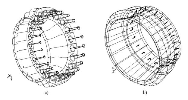
Fig 5. a) Geometry of EV combustor chamber and 30 EV burners with characteristic vortex breakdown [1]; b) Geometry of SEV combustor chamber and 24 SEV burners [1].
