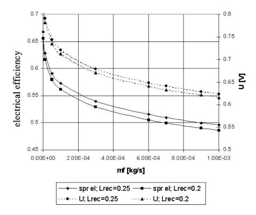
Fig 9. The influence of the recirculation  $L_{rec}$  value on the efficiency and the voltage of SOFC
