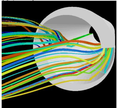
Fig 6. Vortex generation inside EV burners [1,6].
