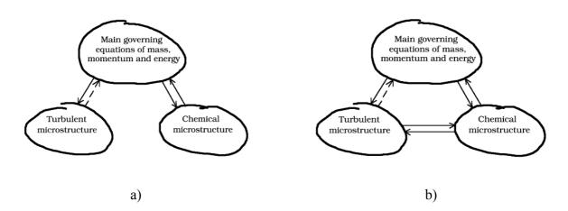
Fig. 2 A scheme of turbulence-chemistry coupling a) classical, b) proposed [3]
