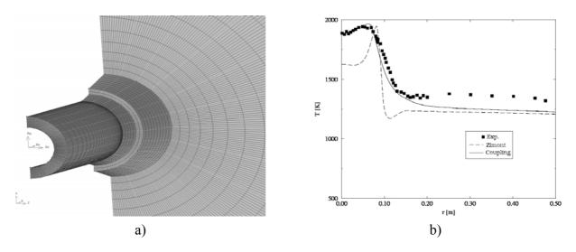
Fig.3. BERL burner, a) the FV discretisation grid details, b) Profile of the temperature at 0.027 m from fuel inlet
