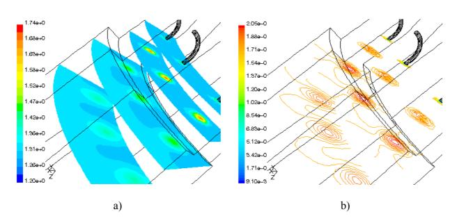
Fig 7. a) Distribution of temperature in SEV chamber; b) Distribution of NO<sub>2</sub> in SEV chamber
