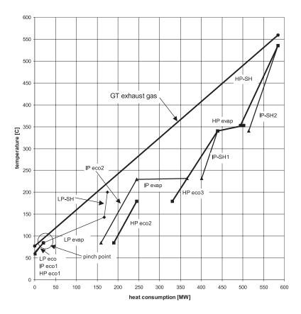
Figure 9. Heat consumption versus temperature diagram for 3PA HRSG at the point of maximum effciency.
