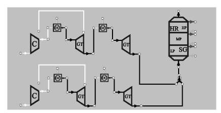
Figure 1. Scheme of combined cycle with the GT26 engine in 2-1-1 configuration.
