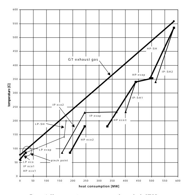
FIGURE 4. Heat consumption versus temperature diagram for the HRSG
