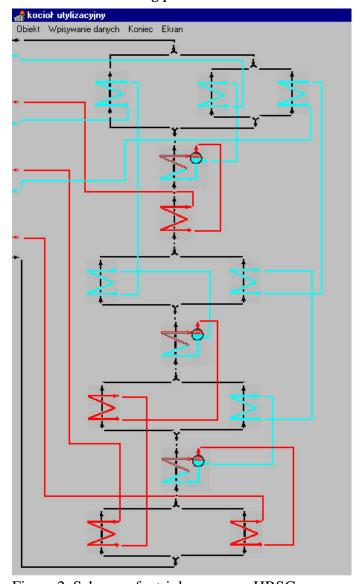
Figure 2. Scheme of a triple-pressure HRSG
