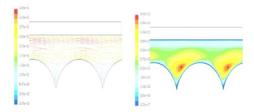
Figure 7. Vectors of velocity of the heated medium at a distance 0.335 m from the inlet to the heated tube.
