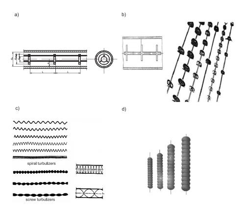
Figure 1. Selected examples of classical turbulizing systems: a) ring inserts [7], b) disk turbulisers [7], c) spiral and screw turbulisers [8, 9], d) ball turbuliser used by authors.
