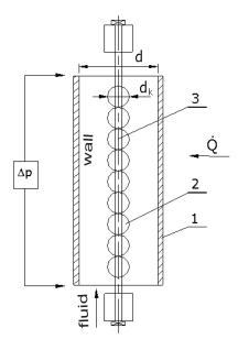
Figure 2. Concept scheme for the ball turbuliser application in a vertical pipe: 1 – vertical pipe with diameter d, 2 – ball turbuliser, 3 – rod placing the turbuliser along the pipe axis.
