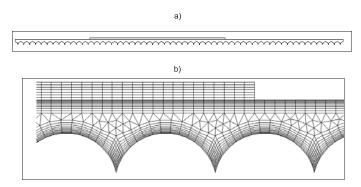
Figure 4. Sketch for copper pipe geometry (a) and fragment of numerical grid with the last heated section (b) .
