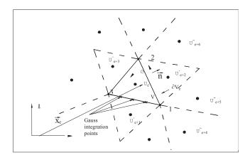
Figure 3. Finite volume  $V_e$  surrounded by its "neighbours" – first rank (with prim  $\mathbf{U'}_{e+n}$ ) and second rank (with bis  $\mathbf{U''}_{e+n}$ ).
