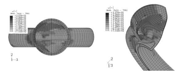
Fig. 9. Damage parameter of HGC after 10000h of operation (Kucharski, 2004)
