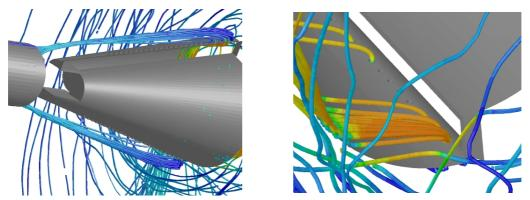
Fig. 2. Particle modeling in EV burner (Badur et al., 2004)
