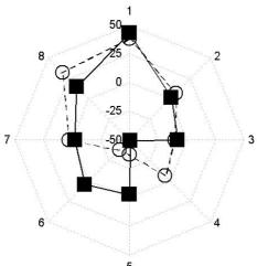
Fig. 6. Circumerential profile of normalized temperature at outlet for operation with closed one of burners ( ○ measurements, ■ computations ) (Badur et al., 2004)
