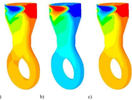
Rys. 7. Case of single burner closing – examplery distribution of : a) temperature, b)  $O_2$  and c)  $H_2O$  (Badur et al., 2004)
