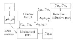
Fig.8. Algorithm of proposed corrosion model. Dashed line represents data obtained from CFD calculations; t – temperature,  $c^{\chi}$  – concentration of chemical species,  $\delta^{ter}$ ,  $\varepsilon^{ter}$  – strains and stresses from thermal loads (Kucharski, 2004)
