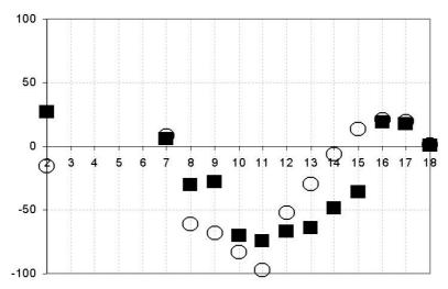
Fig. 5. Normalized temperature changes at turbine outlet for operation with closed burners from 2 to 18 ( ○ measurements, ■ computations ) (Badur et al., 2004)
