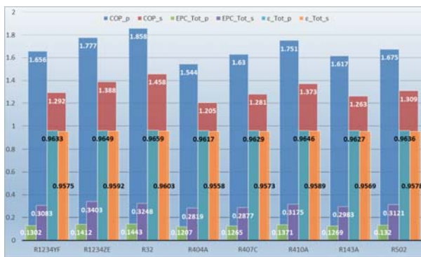
Fig. 2. Variations of COP, EPC & \epsilon objective functions of MRSs and MRSP for different refrigerants
