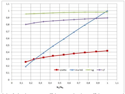
Fig. 3. Characteristic of: electric generators efficiency  $\eta_G$ , electric net efficiency  $\eta_{netto}$ , turbines average mechanical efficiency  $\eta_T$  and live steam mass flow rate  $m_x/m_0$  as a function load variations  $N_x/N_G$  for cycle with steam reheat.
