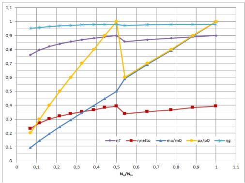
Fig. 4. Characteristic of: electric generators efficiency  $\eta_G$ , electric net efficiency  $\eta_{netto}$ , turbines average mechanical efficiency  $\eta_{T_i}$  and live steam mass flow rate  $m_x/m_0$  as a function load variations  $N_x/N_G$  for cycle with steam reheat.
