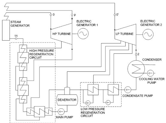
Fig. 2. Steam cycle with reheat thermodynamic scheme
