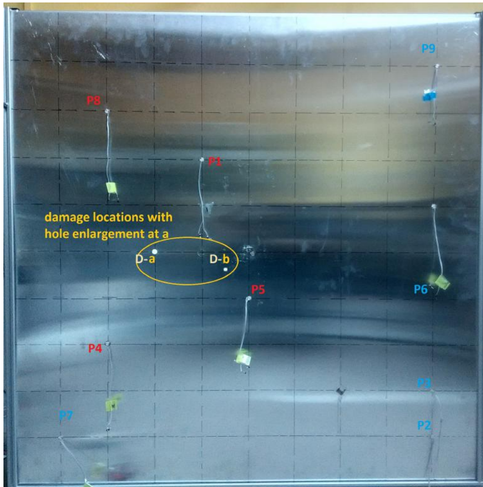
Fig. 3.10 Sensor network distribution against the damage locations in the sample plate.
