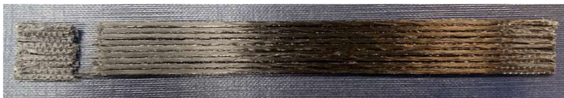
Figure 3.22 Fracture of the sample subjected to sub-zero temperature
