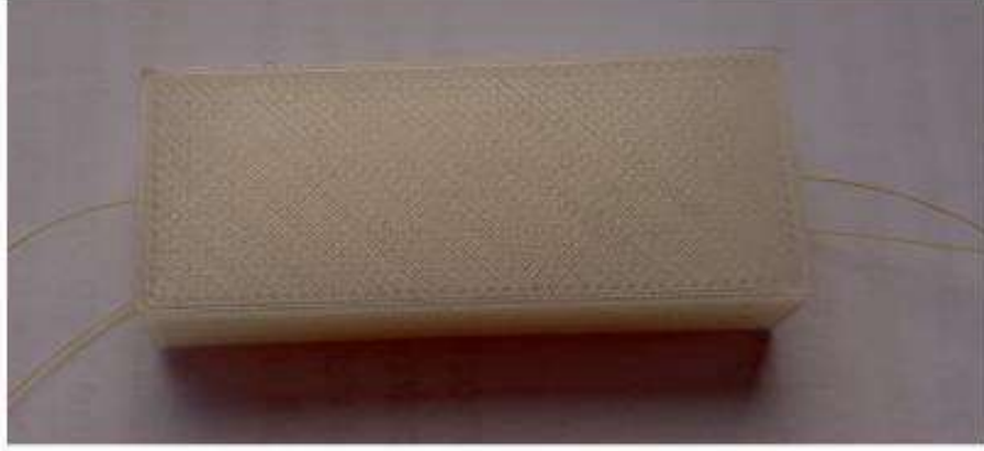
Figure 3.9 PLA sample embedded FBG sensor
