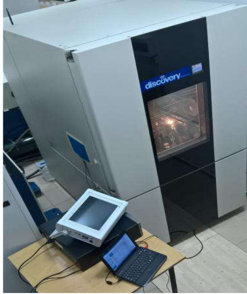
Figure 3.4 MyDiscovery DM600C chamber (IMP PAN laboratory)
