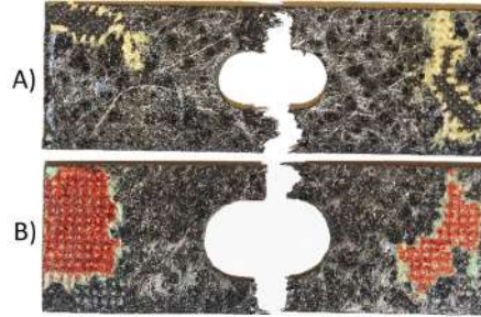
Figure 2.41: Failed fatigue specimens with central hole, A) D=10\text{mm} , B) D=14\text{mm} [149]
