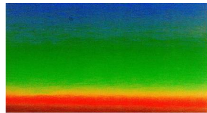
Fig. 6. The distribution of the colour component pattern on the liquid crystal layer measured by RGB colour camera.
