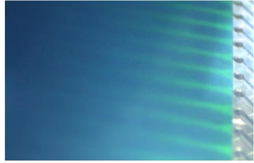
Fig. 27. Visualization of air flow on blade surface. Jet position 1–2, Re = 105\,000 , T_a = 315\text{ K} , T_j = 299\text{ K} , T_{av} = 313.3\text{ K} , \Delta P = 5\% [51].
