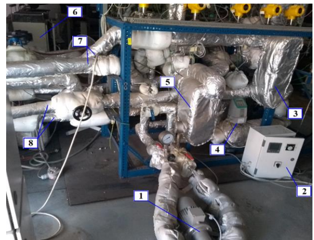
Fig. 3. Micro-ORC power plant test rig: 1 – pumping engine, 2 – frequency converter connected to the PE drive, 3 – evaporator, 4 – Coriolis mass flowmeter, 5 – condenser, 6 – control and regulation module for the induction heater, 7 – heating cycle piping, 8 – cooling cycle piping.
