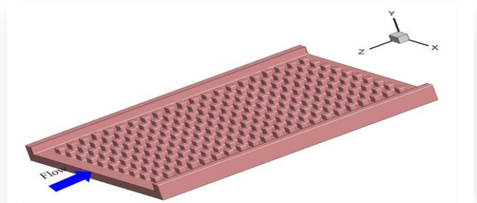
Fig. 1. Isometric view of micro pin fin heat sink.
