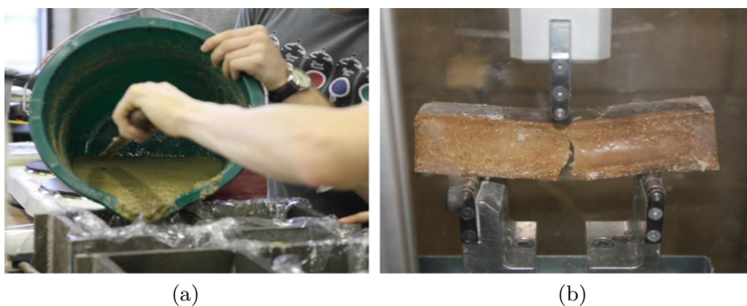
Figure 7: Sample casting (a) and bending test (b) on pykrete specimen [10].
