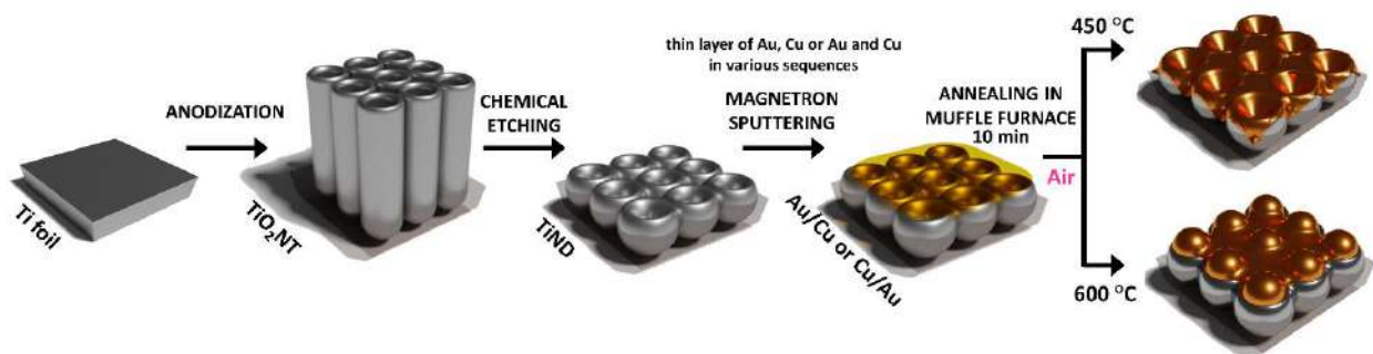
Figure 41. Schematics of fabrication process of AuCu-decorated nanostructured Ti platform.
