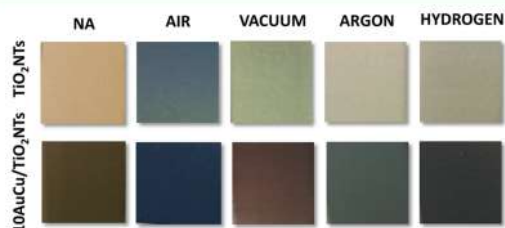
Figure 3. Appearance of TiO 2 NTs and 10AuCu/TiO 2 NTs before and after calcination under different atmospheres.
