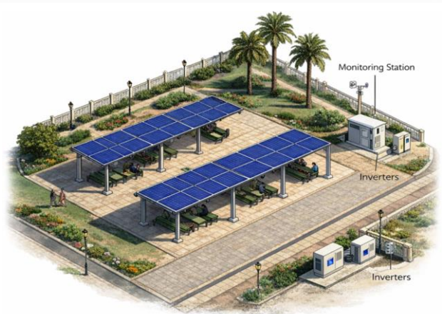
Fig. 2. Schematic configuration of the dual-use photovoltaic canopy system integrated within the public garden, showing the PV module arrangement, supporting structures, and the associated electrical components supplying irrigation and exporting surplus electricity to the grid.
