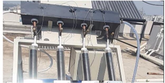
Fig. 5. Experimental setup of evacuated tube solar collector.
