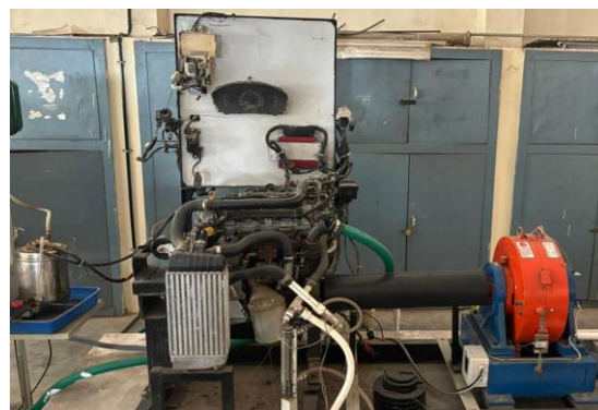
Fig. 7. Common rail direct injection engine setup.
