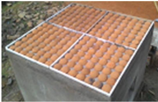
Fig. 3. Earthen pot roof slab model.
