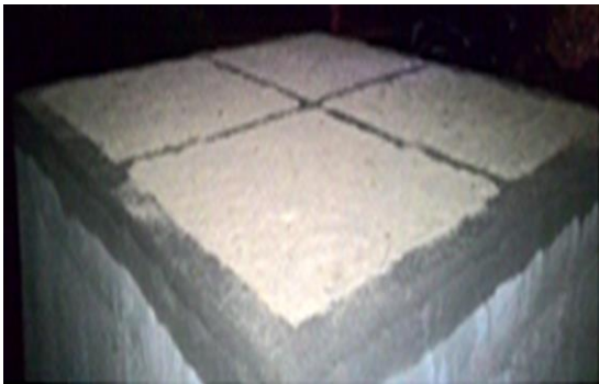
Fig. 4. Rice husk roof slab model.
