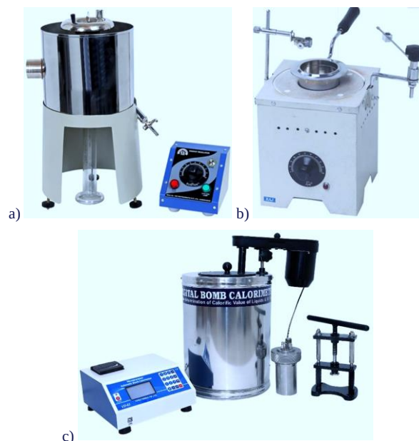
Fig. 3. Redwood viscometer set-up (a), Cleveland set-up (b), bomb calorimeter set-up (c).
