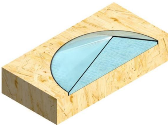
Fig. 2. Schematic representations of the conical solar still design used in the experimental setup, highlighting geometric configuration, materials and insulation layout.
